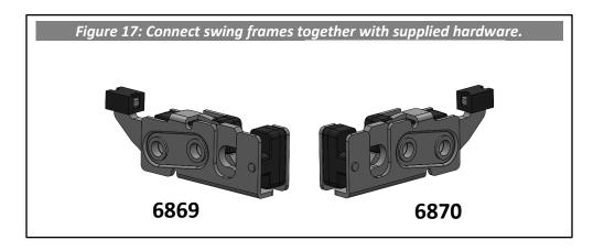
Locate latches and identify using **Figure 17**. Use supplied hardware to install each latch onto swing frame. Latch triggers point outwards from swing frame. Refer to **Figure 18** for hardware order and **Figure 19** for final assembly onto swing frame. **Following this order is crucial to preventing damage to components**. Torque latches to **10 ft-lbs**.
