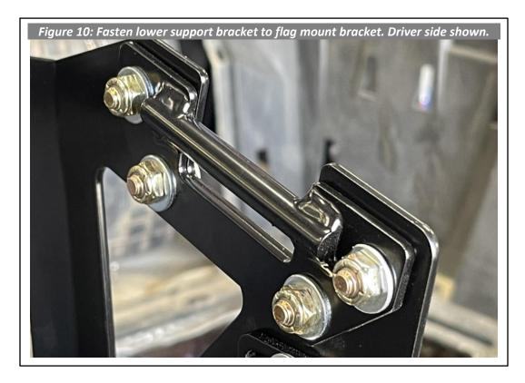
**10.** The spare tire lower support assembly is complete. Torque hardware to following:
