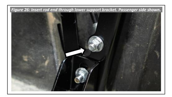
Holding the rod ends with a **13mm** wrench, use a **1/2**" socket to torque the four lock nuts to **8 ft-lbs**. Lower and latch the swing frame. Place a tire or a weight of around 80 lbs on the spare tire carrier. Unlatch and raise the swing frame. The gas struts should be able to independently support the swing frame and weight.
