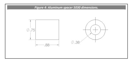
Clean any debris from bedliner pockets. Place one 5030 spacer into each pocket in the bedliner. Pass M6 bolts through 1/4" washers, foot brackets, then spacers, and thread into chassis. Orient foot bracket as shown in **Figure 5**. Long slot should be vertical. Tighten until secure but do not torque.
