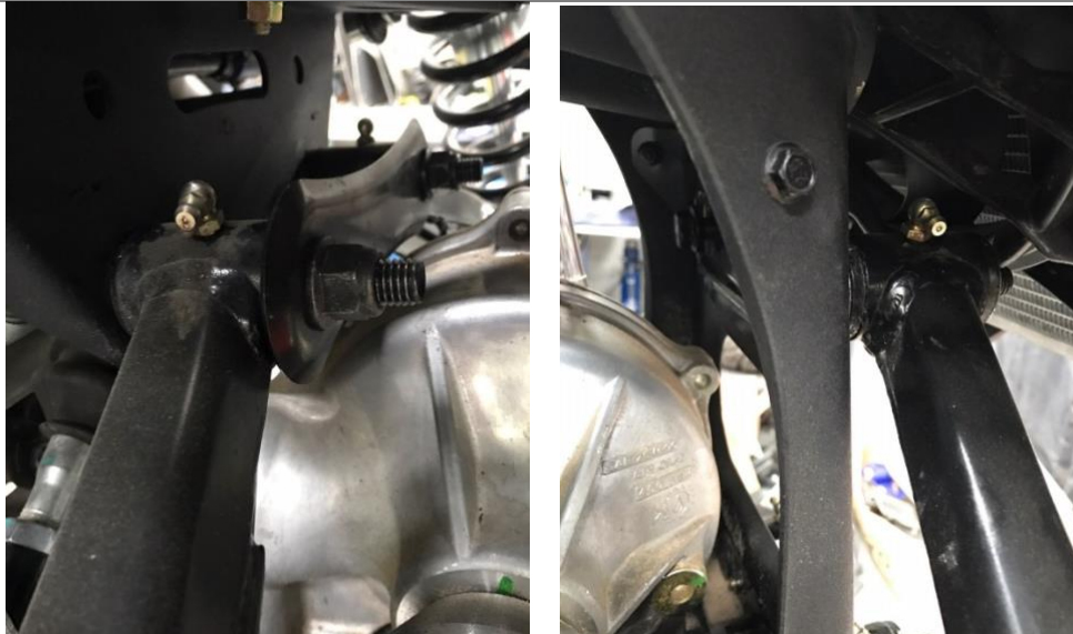
Figure 1: Remove nuts off pivot bolts
