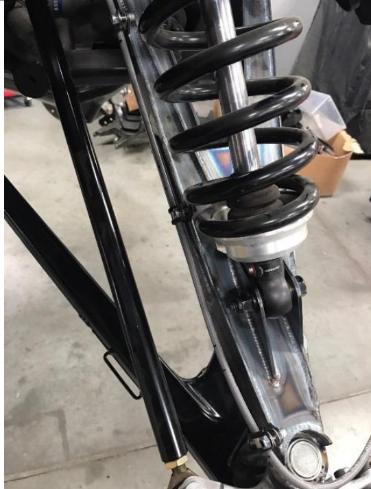
Figure 5: Brake line routing
