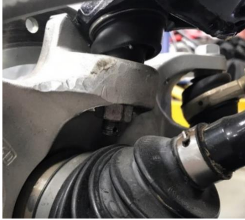
Figure 1: Remove nut and washer off bottom side of ball joint
