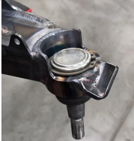
Figure 3: Ball joint pressed into Cognito arm.
