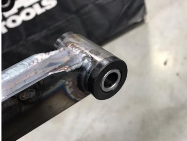
Figure 4: New bushings and crush sleeves in pivot tubes
