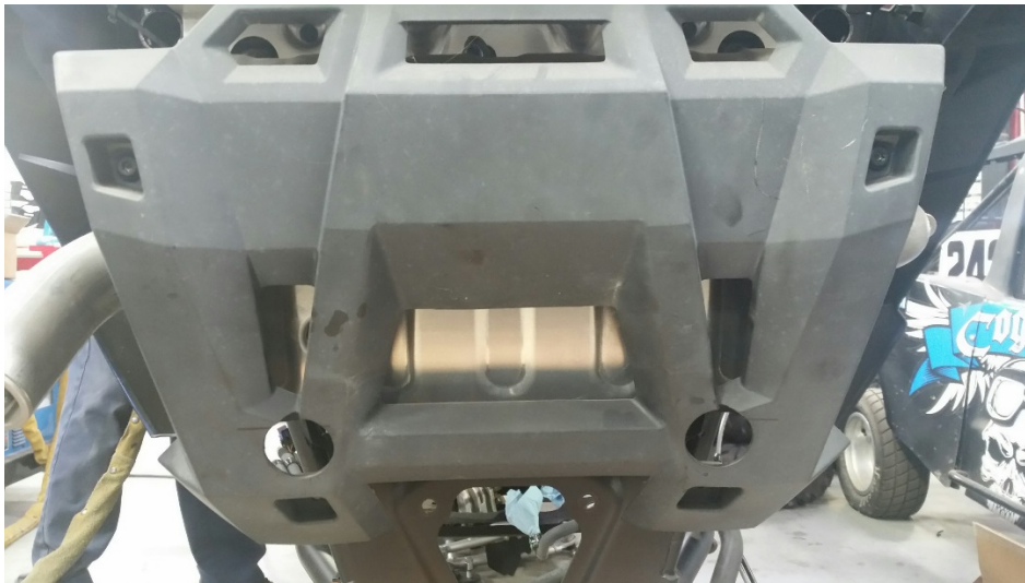
Figure 2: The plastic OEM rear bumper hole sawed and attached.
