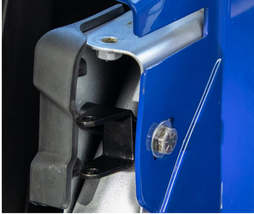
Figure 4b: Limit Strap Bracket Installed
