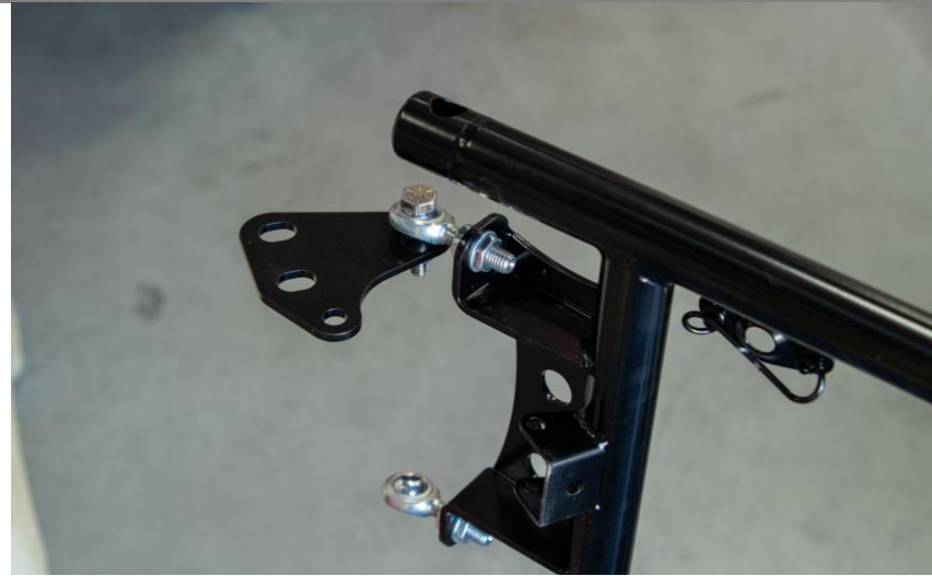
Figure 6: Upper Hinge Plate Installed on Driver's Side
